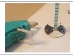
6. Use hot glue to attach the bottom of the straw to the center of the painted side of the washer.
