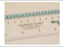
5. Line up the bottom of the straw with the 0 cm mark and use a marker to make a mark every 0.5 cm along the straw.
