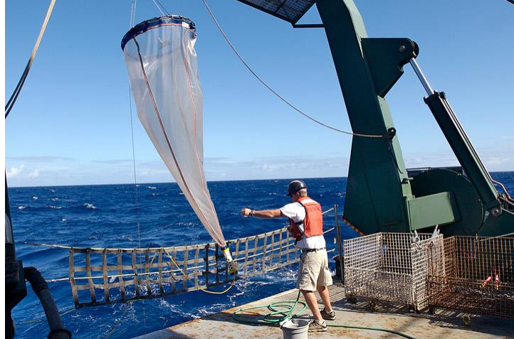
Marine biologists use plankton nets to sample phytoplankton directly from the ocean (Photograph ©2007 Ben Pittenger)
