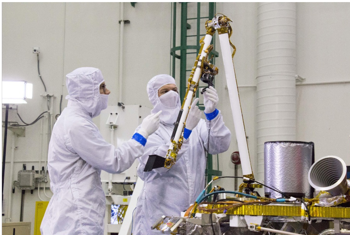
NASA/JPL-Caltech/Lockheed Martin Space. (n.d.). Pre-launch testing of InSight's robotic arm. NASA. https://www.jpl.nasa.gov/spaceimages/details.php?id=PIA22741
